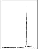
Figure 9: CE of a Poly-Pak purified biotinylated oligonucleotide, following the conditions shown in Figure 2, Page 15.
