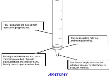
OF A OF A POLY-PAK™ BARREL
