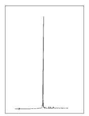
Figure 3: RP HPLC of an amino-modified oligonucleotide purified as described. Column, flow rate and detector are as described in Figure 1, Page 15.
