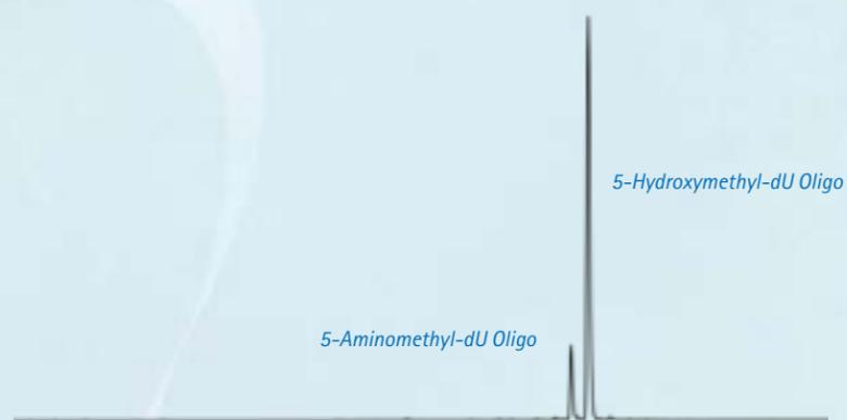
FIGURE 3: RP HPLC OF 5-HMDU-T6 OLIGO DEPROTECTED WITH AMA AT 65° C
