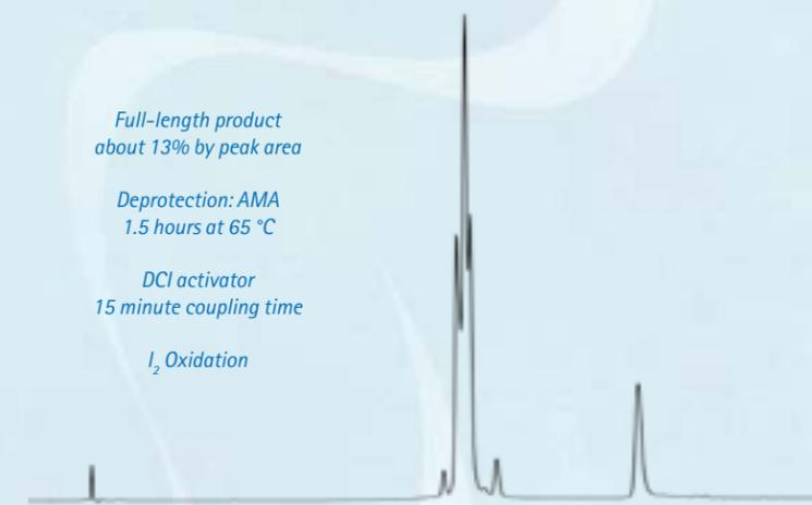
FIGURE 3: RP HPLC OF A MIXED BASE 16MER WITH 6 ADDITIONS OF 2-AMINO-dA AND CSO OXIDATION
