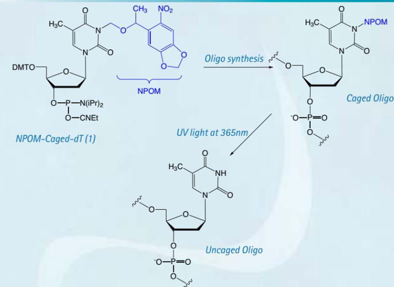
FIGURE 2: STRUCTURE OF NPOM-CAGED-dT
