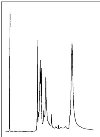
**Figure 6:** RP HPLC of a crude oligonucleotide modified at the 5' terminus with thiol-modifier C6 S-S following the conditions shown in Figure 1, Page 15.
