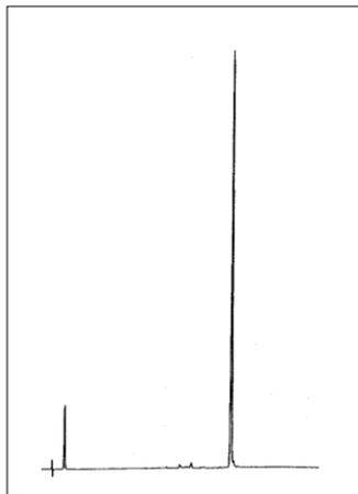
**Figure 11:** RP HPLC of a Cy-3 labelled oligonucleotide, following the conditions shown in Figure 1, Page 15.
