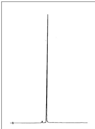
**Figure 10:** RP HPLC of a FAM labelled oligonucleotide, using the conditions shown in Figure 1, Page 15.
