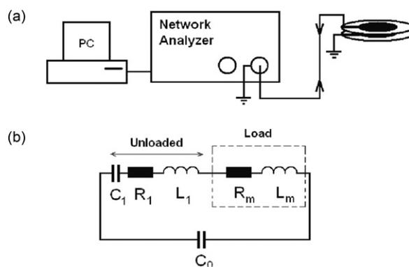
**Fig. 1** (a) TSM experimental setup,<sup>23</sup> and (b) Butterworth van Dyke (BVD) model for the electrical circuit of the quartz crystal transducer.<sup>22</sup>
