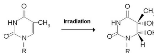
**Scheme 1** Transformation of thymidine to thymidine glycol under the action of ionizing irradiation. Only one *cis* (5*R*,6*S*) isomer from four possible epimers was used in this study.
