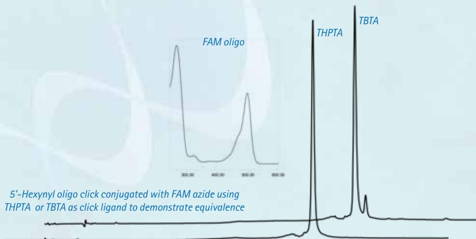
FIGURE 4: RP HPLC ANALYSIS - 1 μMOLE AQUEOUS REACTION WITH FAM AZIDE AND THPTA, 30 MINUTES
