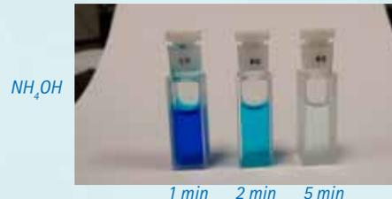
5'-Cyanine 5 labelled T12 oligonucleotides were synthesized on Glen UnySupport and Glen UnySupport FC. Each support was deprotected with AMA or ammonium hydroxide. The supernatant was removed and transferred to a cuvette and fresh solution was added to the support. The total exposure time of each sample is shown.
